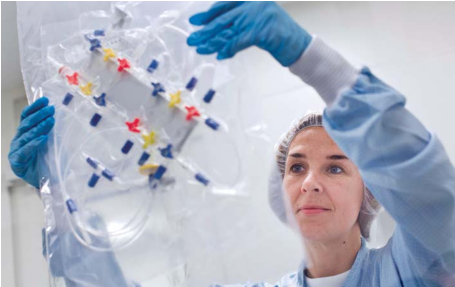
Check of a synthesis cassette for a modular lab
